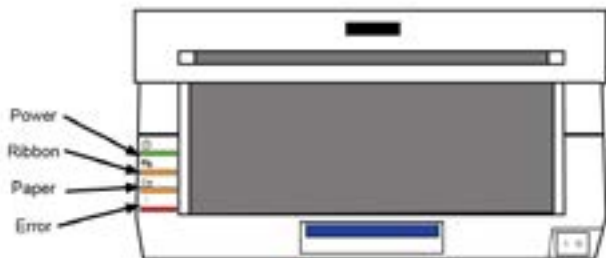
The status of the LED indicates the Printer Status
